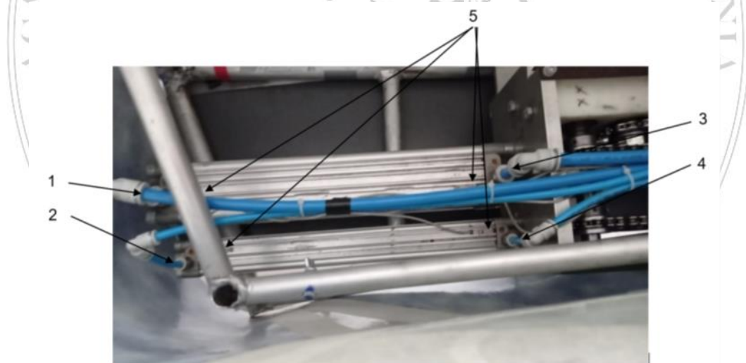
Fig. 7. Image of the sensors mounted at the ends of the cylinders
