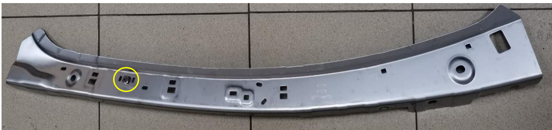
Fig. 5. Semi-finished product 1 with welded nut.
