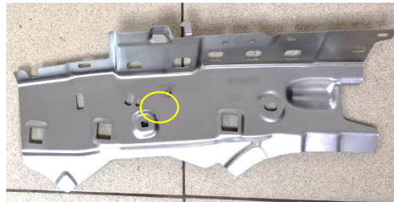
Fig. 10. Semi-finished product 4 with welded screw.
