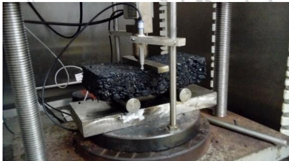
Fig. 5. Mixture reinforced with geocomposite – cracked without broke
