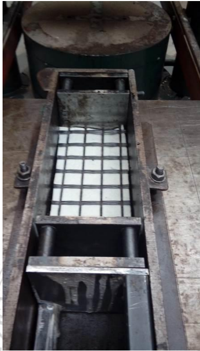
Fig. 2. Preparing the bituminous mixture with geocomposite.
