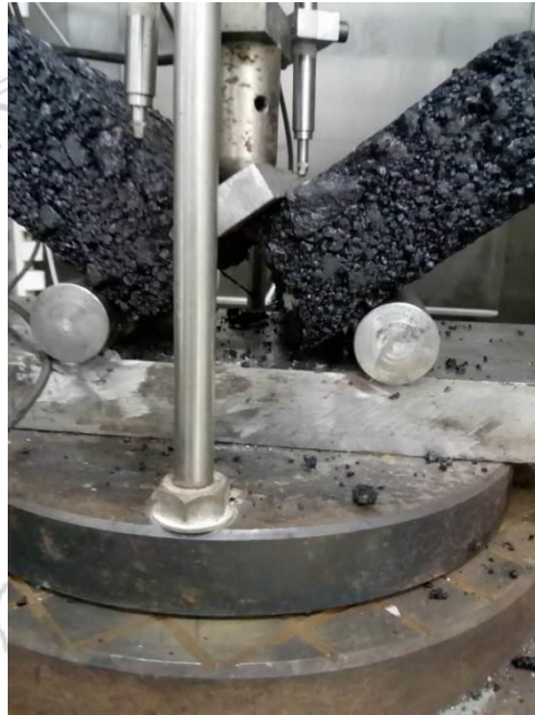
Fig. 4. Normal mixture specimen – cracked and broken.
