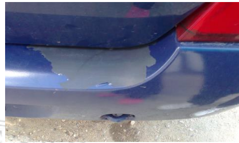
Fig. 14. Rear paint bark peeling
