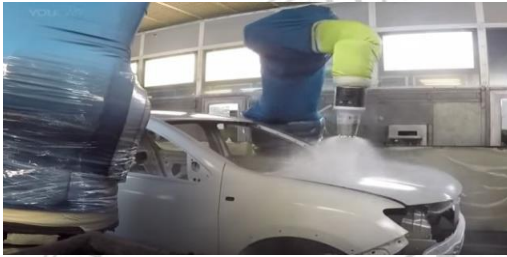
Fig. 8. Application of protection lake [5]
