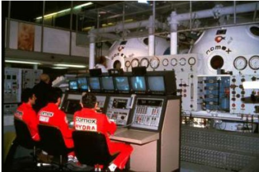
Fig. 1. Hyperbaric chambers belonging to the system for simulation diving with hydrogen-based mixtures at C.E.H. COMEX in Marseille.
