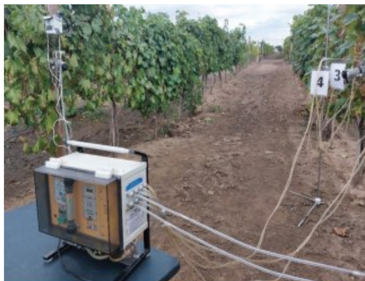
Fig.4 Phytomonitor for determining physiological indices in plants
