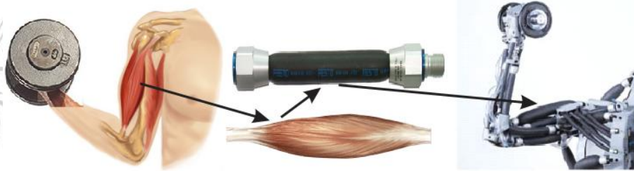
Fig. 6. Pneumatic artificial muscles mimic a biological muscle
