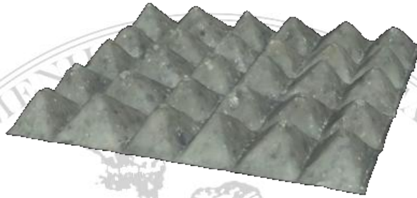
Fig. 1. Portion of new TRIZACT 307EA belt.
