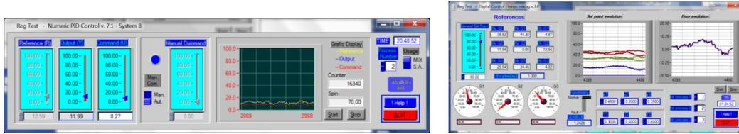
**Fig. 14.** a) single closed loop PID controller; b) proposed control structure (variant solution).
