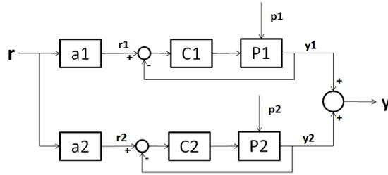
**Fig. 2.** Classic solution based on parallel connection of two or more sources without compensation.
