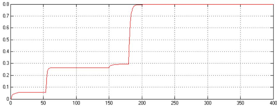
**Fig. 8.** Absolute integral error evolution for two parallel systems with compensation.
