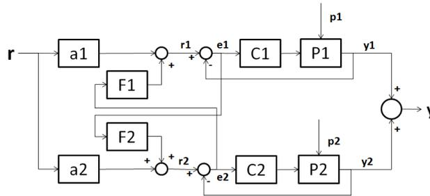
**Fig. 5.** The proposed solution for a parallel connection of two sources with balance structure.
