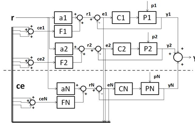
Fig. 9. The proposed solution for a parallel connection of N sources with balance structure.
