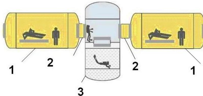
**Fig. 1.** Hyperbaric Complex: 1) dry hyperbaric chamber, 2) sas, 3) wet hyperbaric chamber.
