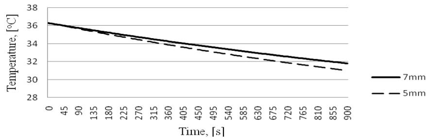
**Fig. 7.** Body temperature variation for the diver 3, at 30 m depth, for two different thickness of the neoprene wet suit: 5 mm and 7 mm.
