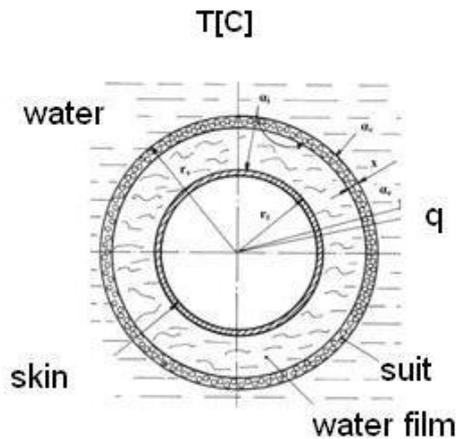
**Fig. 2.** Heat transfer by ensemble human body-skin-water film-suit-water.
