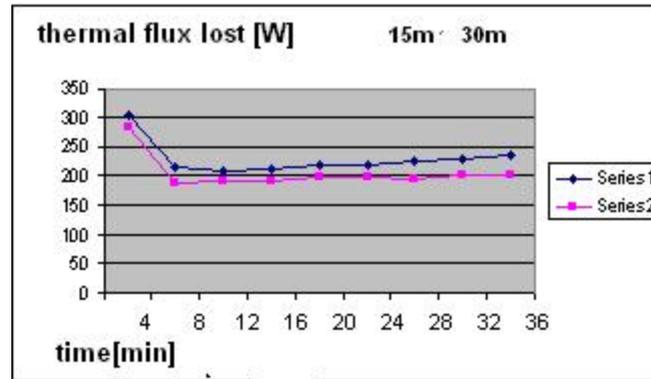
**Fig. 6.** Lost thermal flux variation [ $\text{W}/\text{m}^2$ ] by diver 1, in time, at 15 m and 30 m depth.
