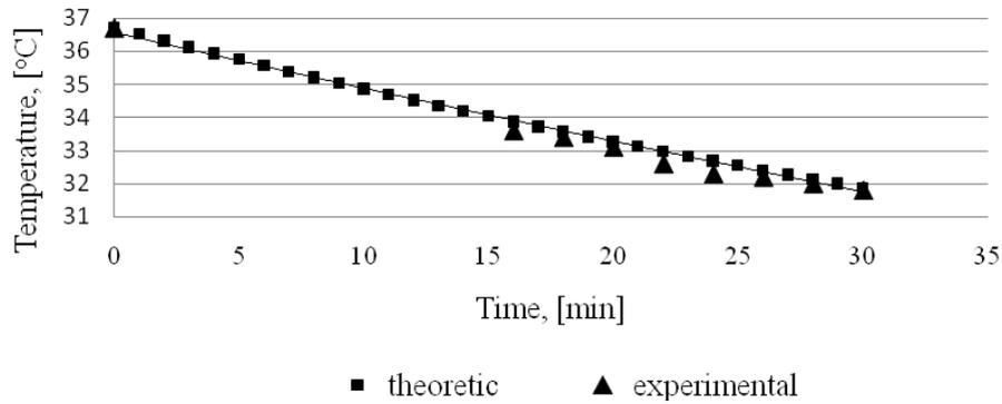
**Fig. 5.** Body temperature variation for the diver 2, at 30 m depth, wearing a 5 mm neoprene wet suit. Theoretic and experimental curves,  $R^2 = 0.8$ .
