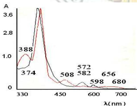
**Fig. 2.** The UV VIS spectra of  $(\text{TPP-Mn})_2\text{-O}$  and TPP-MnCl (insert)
