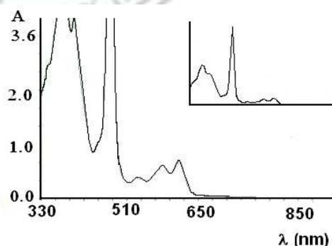
**Fig. 3.** Comparative UV-VIS spectra of  $(\text{TPP-Fe})_2\text{-O}$  (continuous line) and TPP-FeCl (interrupted line)
