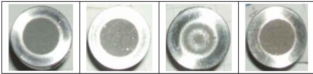
Fig. 5 Aspects of the eroded specimens.
