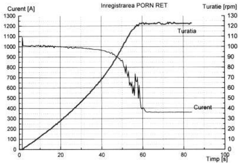
**Fig. 2.** Current and speed at start in asynchronous conditions at reduced voltage of a 13880 kVA reversible synchronous hydrogenerator.
