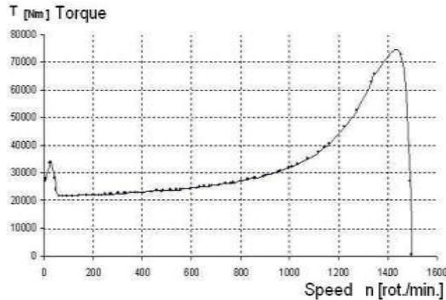
Fig. 6. Torque speed characteristic of a 5250 kW induction motor obtained with EMTS
