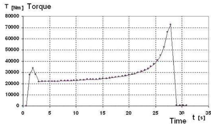
**Fig. 5.** Torque as time function, at slowly starting conditions of a 5250 kW induction motor.
