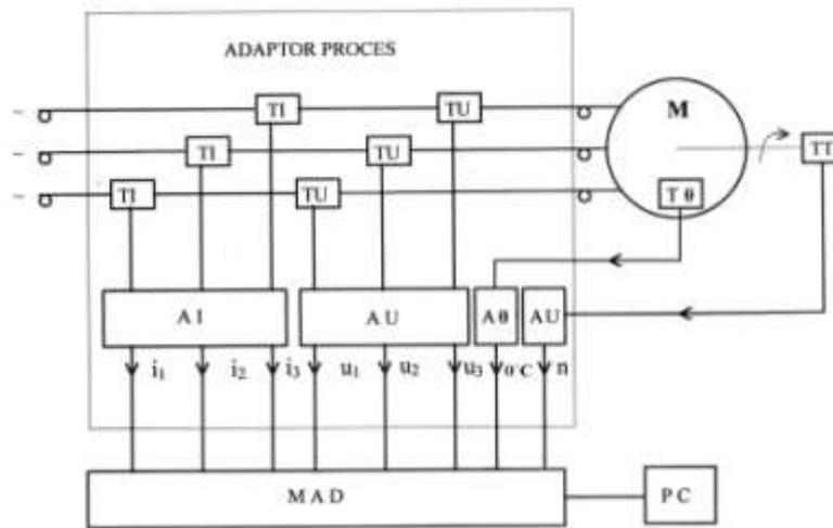
**Fig. 1.** Bloc diagram of DAPS in a measuring circuit.
