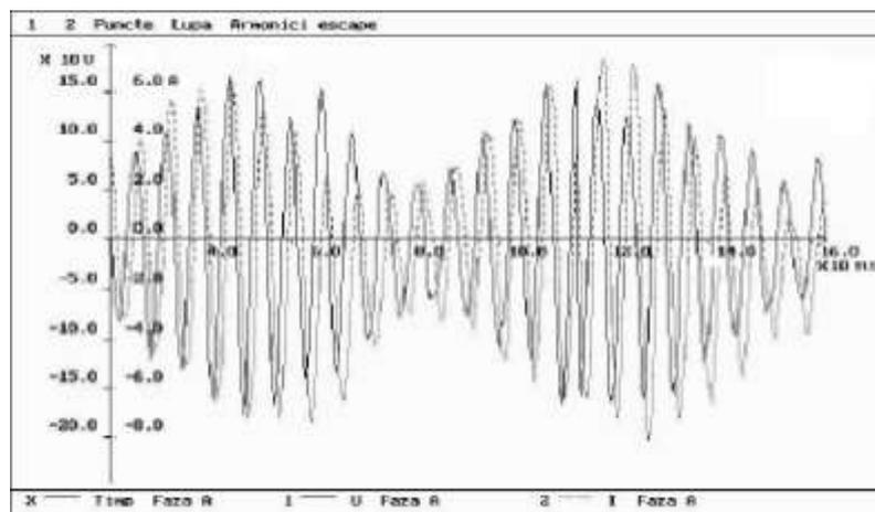
Fig. 7. Wave form of voltage and current per phase in mixed frequency test of an induction motor.
