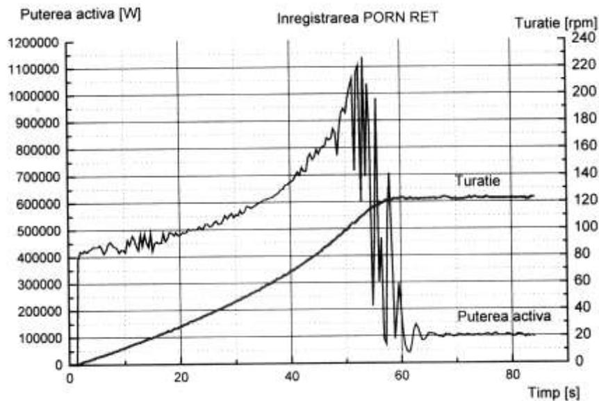
**Fig. 3.** Active power and speed at start in asynchronous conditions at low voltage of a 13880 kVA reversible synchronous hydrogenerator.
