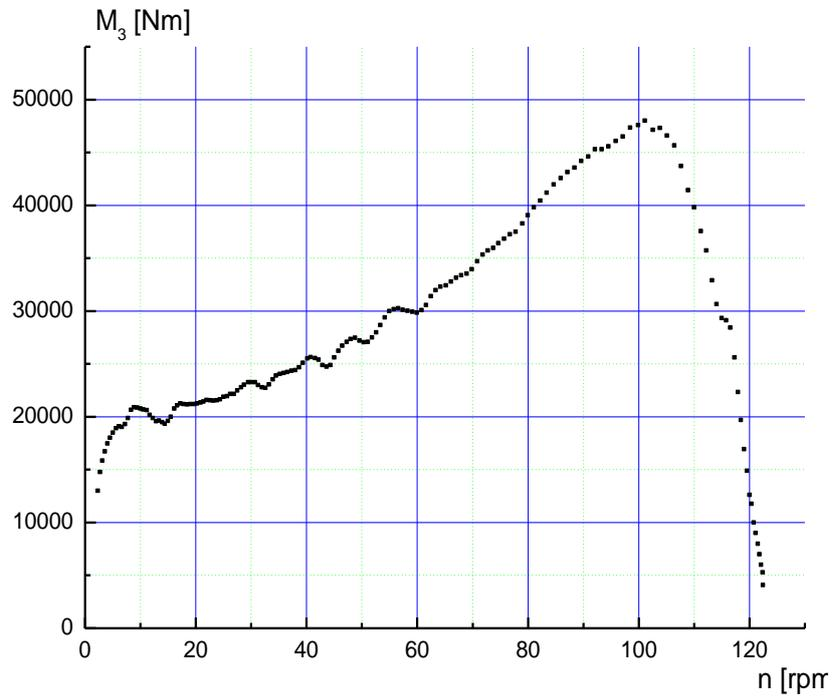
**Fig. 4.** Torque characteristic from starting at low voltage test.
