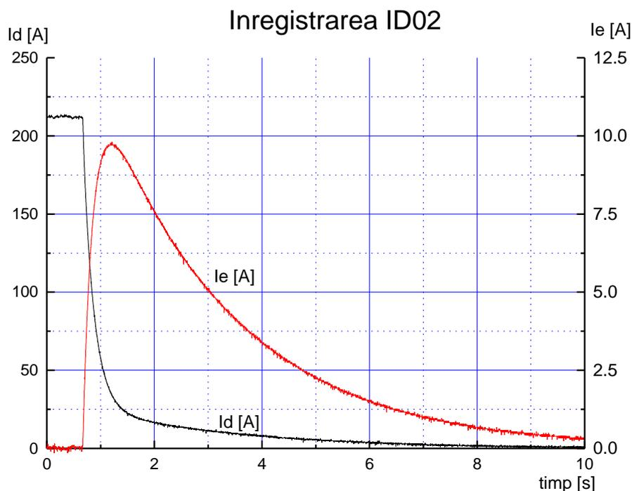
**Fig. 8.** Example of field current  $i_e$  and longitudinal current  $i_d$  in a d.c. decay test
