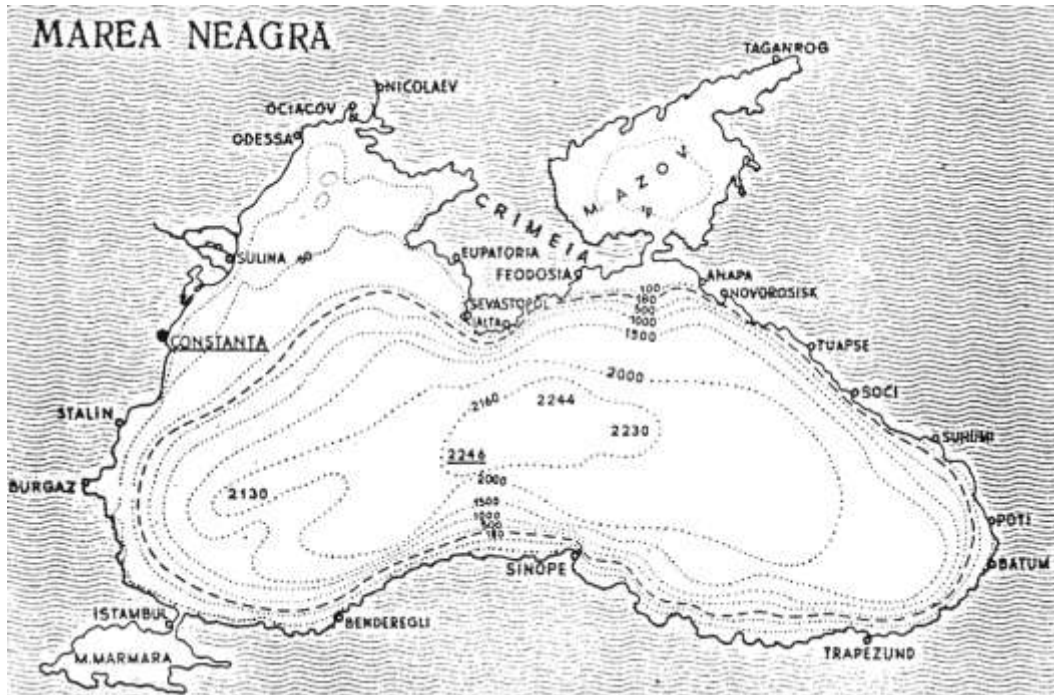
Fig. 5. The aspect of isobathic lines in the Black Sea, the 180 m isobath marking the deep zone contaminated with hydrogen sulphide
