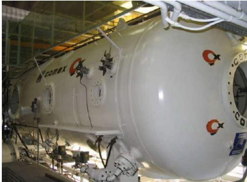
Fig. 4 Hyperbaric chamber used for HELIOX diving, part of the hyperbaric complex at the COMEX Hyperbaric Test Center in Marseille.
