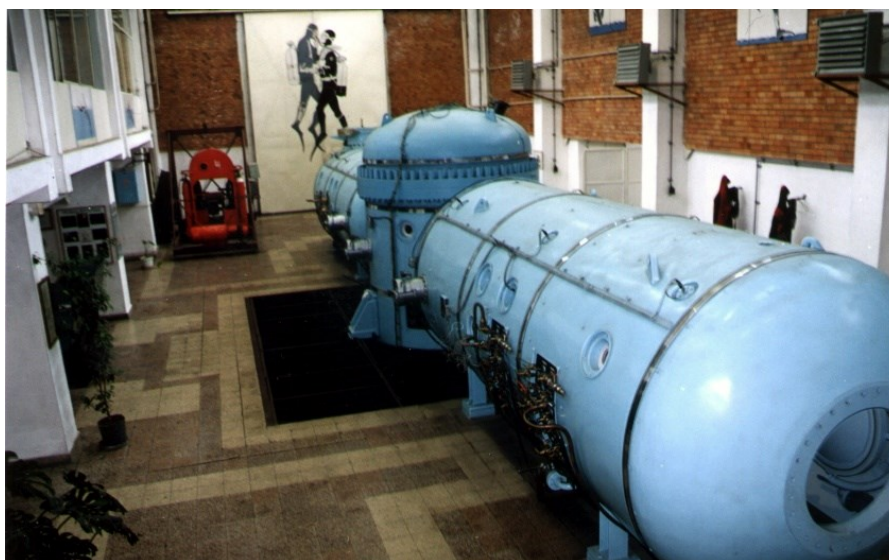
Fig. 6. The hyperbaric system used by the Hyperbaric Laboratory at the Constanța Diving Center.
