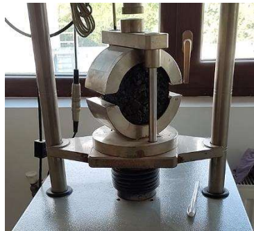
Fig. 3. Littar specimen in Marshall stability test clamp
