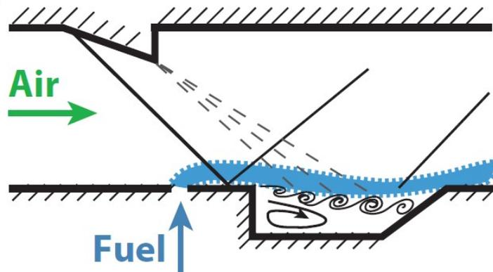
Figure 1. Cavity flow for supersonic combustion [1]
