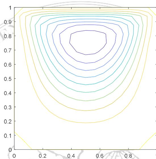
Figure 5. Streamlines inside the cavity flow
