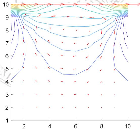
Figure 6. Velocity field and streamlines inside the cavity
