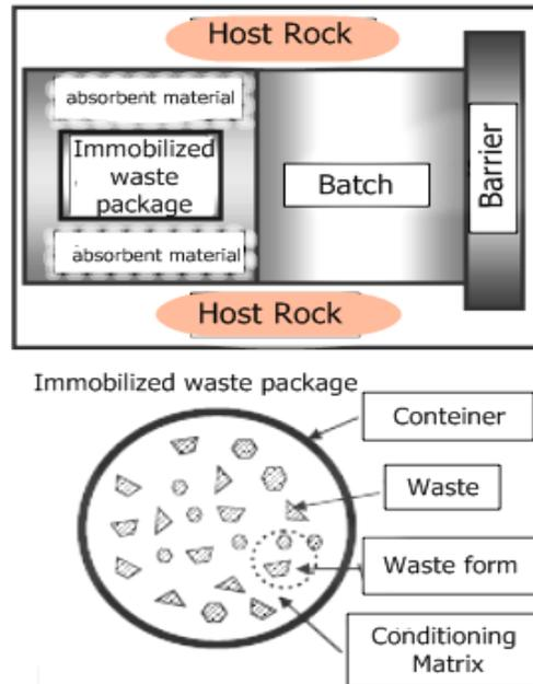
**Fig. 5.** Components of the storage system.
