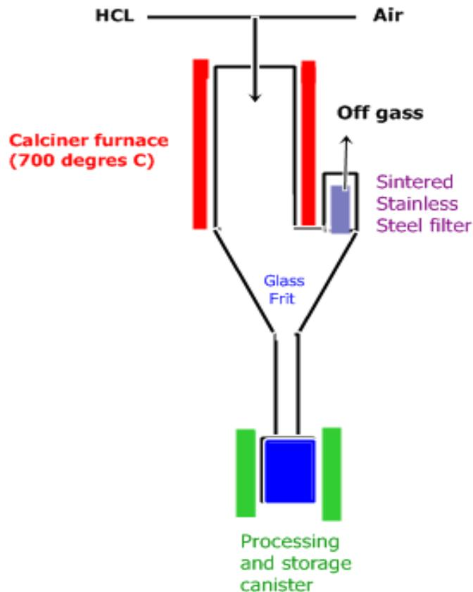
**Fig.3.** Example of the vitrification process is a technique called "In-Can-Melter"
