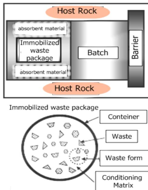
**Fig. 5.** Components of the storage system.
