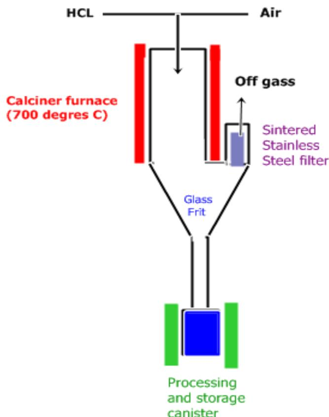
**Fig.3.** Example of the vitrification process is a technique called "In-Can-Melter"
