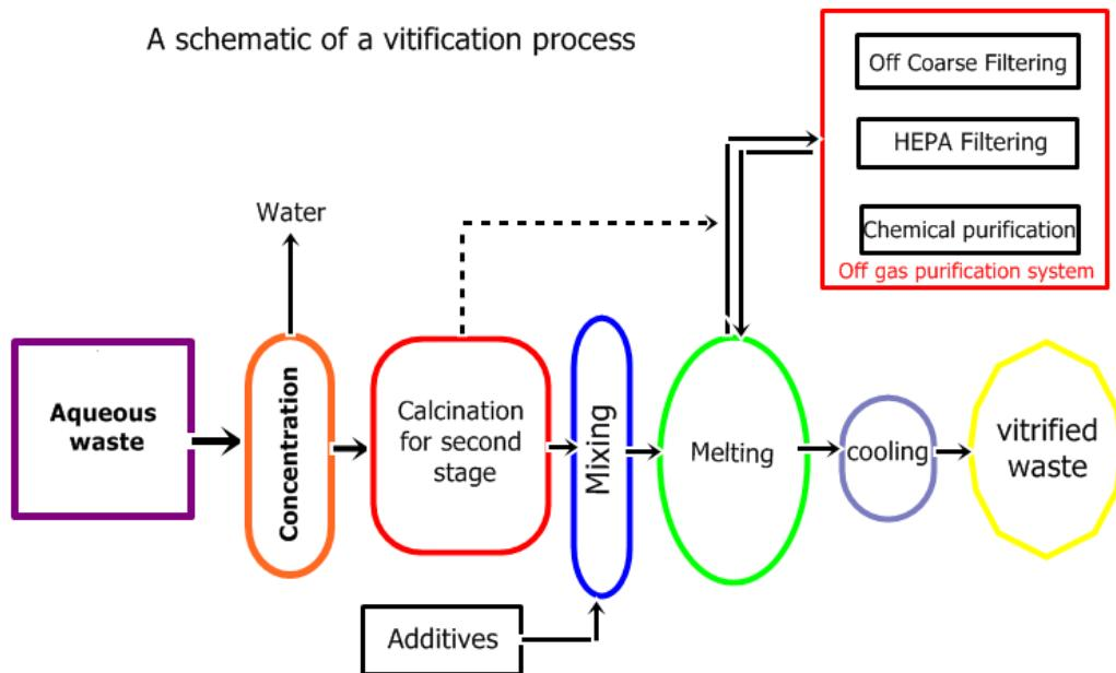
**Fig.4.** A schematic of vitification, using borosilicate glass.
