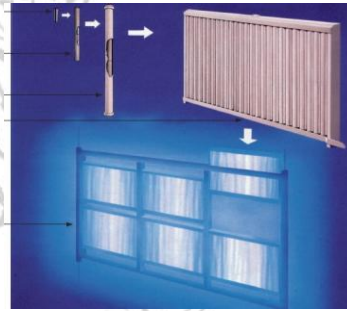
Fig. 3. A typical cobalt source rack.
