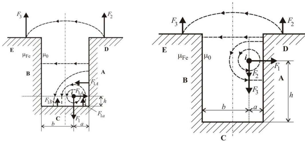
**Fig. 3.** Electric conductor placed inside a ferromagnetic slot.
