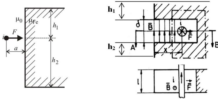
**Fig. 1.** Electric conductor placed close to a massive ferromagnetic piece, as described:
