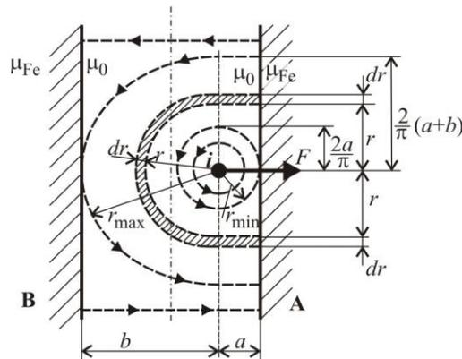
Fig. 2. Electric conductor placed between two ferromagnetic walls.
