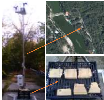
Fig. 4. Exposure place for samples C1÷ C6 near shore of Ciric Lake, with geographical coordinate: 47.182827 N, 27.604205 E.
