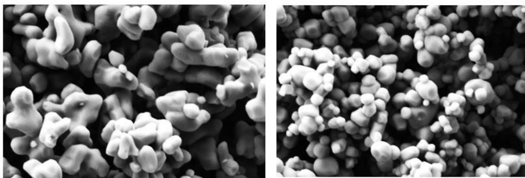
**Figure 9.** AFM images of 588+TiO<sub>2</sub> non-irradiated (left) and after irradiation (right) - 1x1 μm – mod contact
