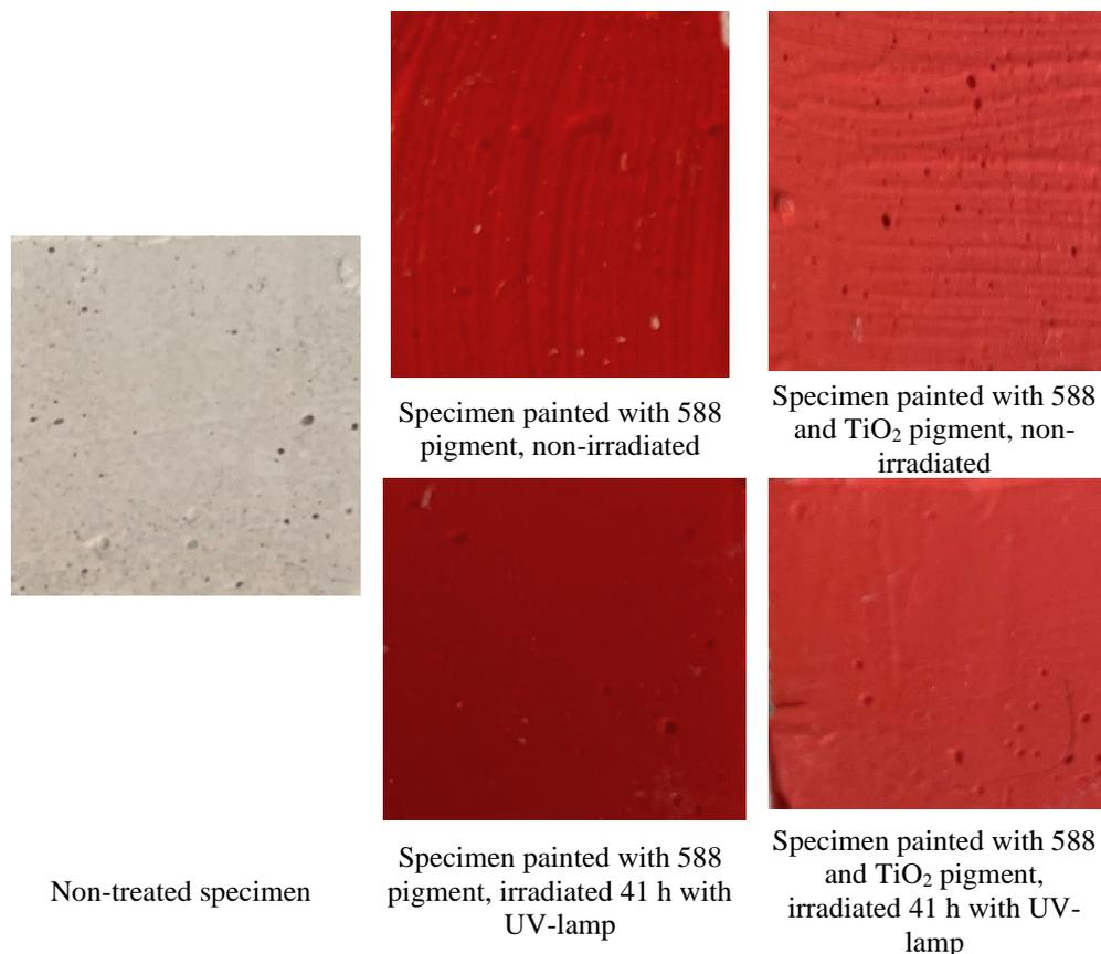
**Figure 7.** The optical microscopy of the painted specimens with 588 (naphthol red with diaryl yellow) pigments
