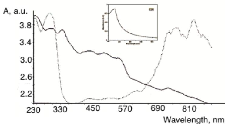
**Figure 2.** UV-Vis spectra of 588 painting paste: non-irradiated with UV light (\_\_\_\_) and irradiated 41 h with UV light (.....) (TiO<sub>2</sub> spectrum inset)
