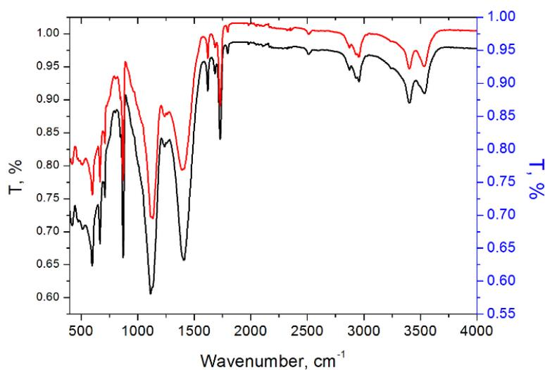
**Figure 3.** FTIR of 588+ $\text{TiO}_2$  layer: non-irradiated (black) and irradiated 41 h (red)
