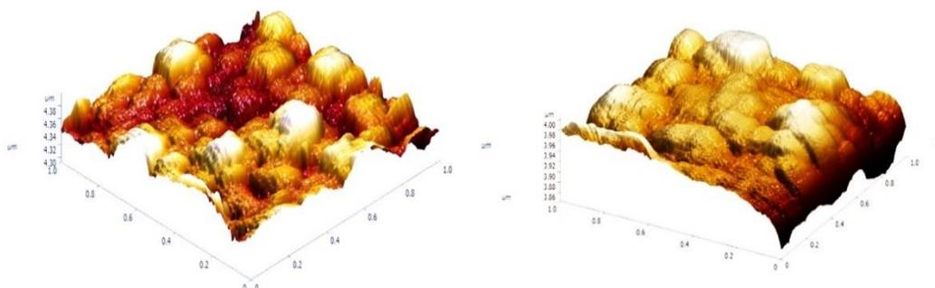
**Figure 8.** SEM of the painted surface: before (left) and after (right) irradiation
