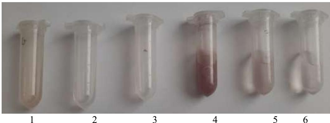
**Fig. 1.** Photo of solutions of GaSe nanosheets in water (1, 2, 3) and acetone (4, 5, 6) obtained by ultrasonic fragmentation. Samples (1) and (4) were prepared without centrifugation, while samples (2) and (5) were centrifuged at 3500 rpm, and samples (3) and (6) at 7000 rpm.
