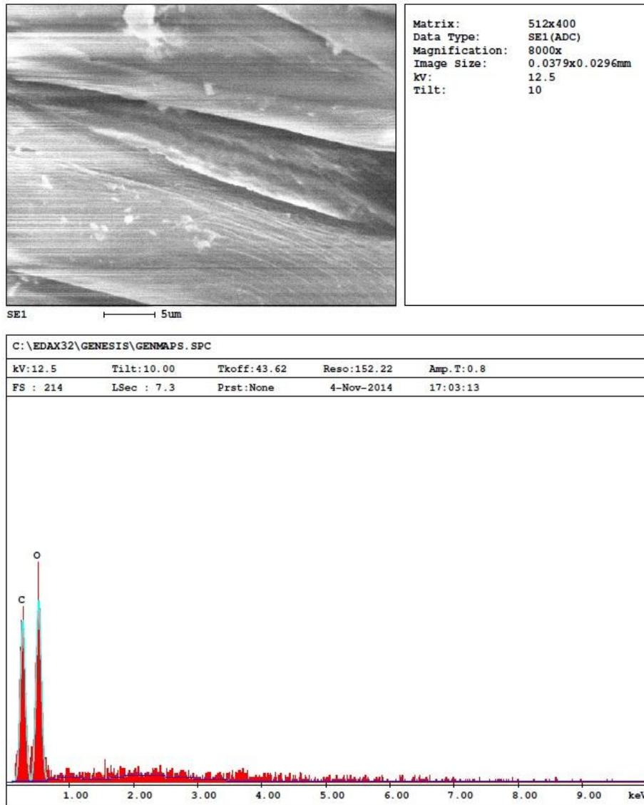
**Fig. 1.** Hydrophilic cotton – before fluorocarbon plasma treatment.
