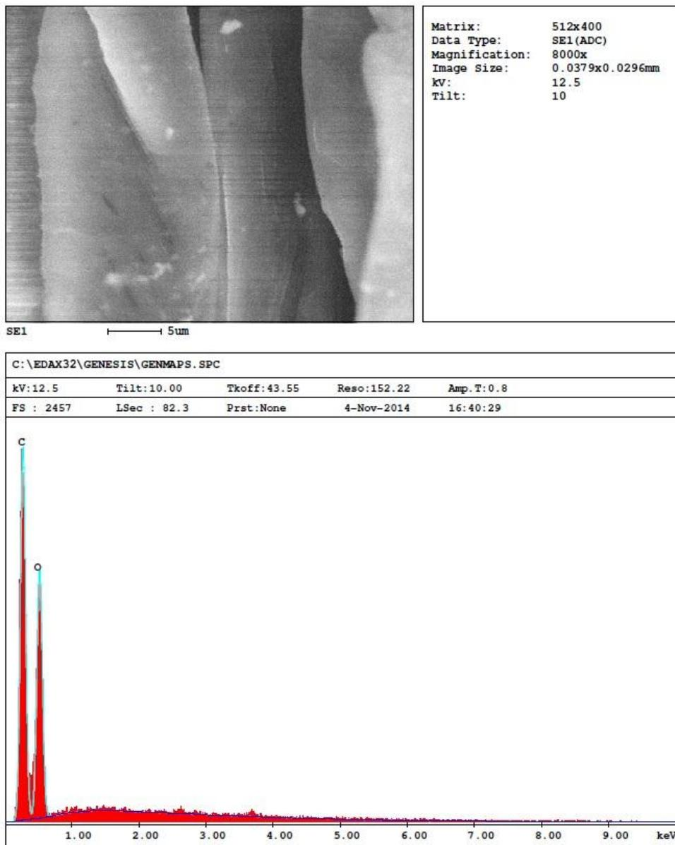
**Fig. 2.** Hydrophobic cotton - after fluorocarbon plasma treatment.
