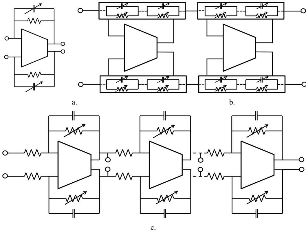
Fig. 3 – The modular architecture of the SDRRX LF blocks
