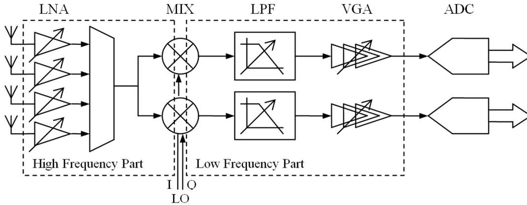
Fig. 1 – Generic SDRRX block diagram [1].
