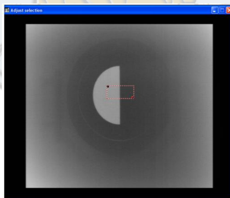
Fig. 9. Original Image for measurement MTF (aligned focal lens 135 mm) with DT 1500 tester thermal camera and related software from Inframet.
