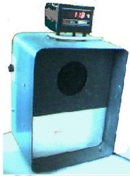
Fig. 9. The black body Wahl standard source, with the characteristics: • Temperature domain: 0-350 °C; • Constant of temperature: 2 °C; • Aperture diameter: 100 mm.
