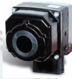
Fig. 11. A view of PathFindIR thermal camera with next characteristics: • Spectral domain: 8-12 μm; • Radiometric resolution: 8 bits; • Visual field: 40°H×30°V); • Geometric resolution: 6,6".
