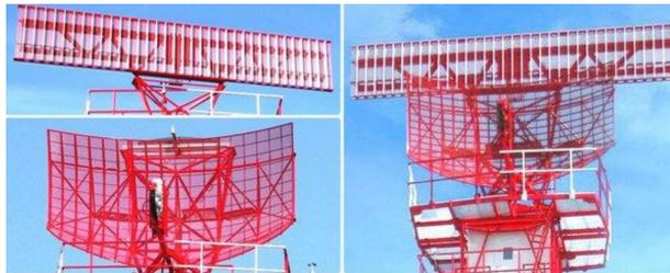
**Figure 1.** Airport antennae for SSR (left side top) and PSR (left side down).
