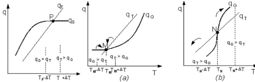
Fig. 2. Geometrical stability analysis in  $q-T$  diagram
