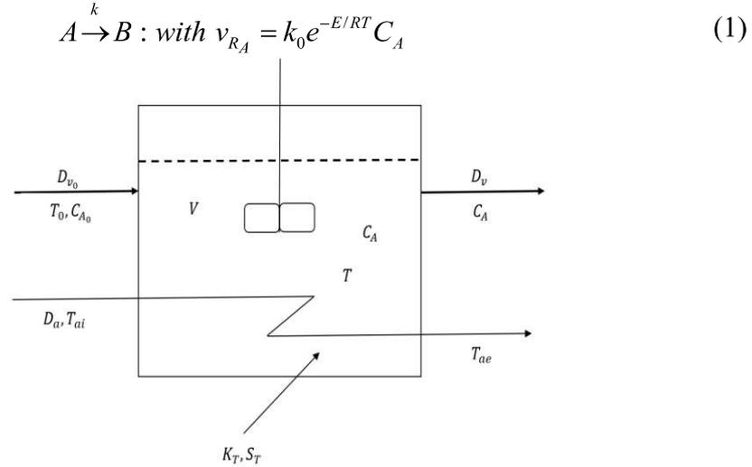
**Fig. 1.** Non-isothermal Continuous Stirred Tank Reactor- NCSTR
