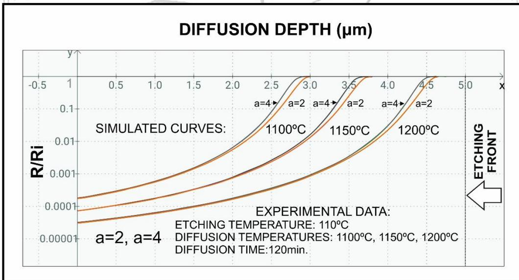
**Fig. 5.** Comparative analysis of R/Ri ratio during the chemical etching process of the boron diffused silicon layers in  $a=2$  and  $a=4$  type etching solutions, simulated according to the analytical results describing the boron profile after the diffusion from the BN source at  $1100^\circ\text{C}$ ,  $1150^\circ\text{C}$  and  $1200^\circ\text{C}$  for 120min. The temperature of the etching solutions is  $T_e = 110^\circ\text{C}$ .
