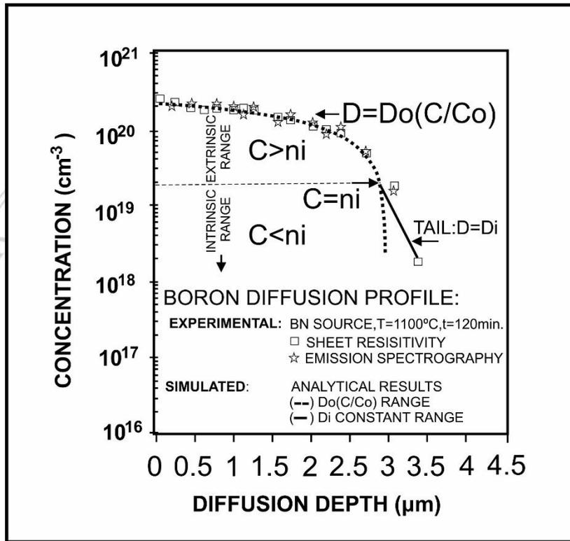
**Fig. 1.** Boron diffusion profile in silicon experimentally determined by electrical (sheet resistivity) method and by chemical (emission spectrography) and simulated (dashed and full line) after the diffusion from a BN source at 1100°C for 120min.
