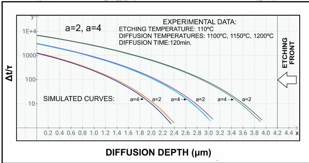
**Fig. 6.** Comparative variation of the etching time expressed as the ratio  $\Delta t/\tau$ , during the chemical etching process of the boron diffused silicon layers in  $a=2$  and  $a=4$  type etching solutions, simulated according to the analytical results describing the boron profile after the diffusion from the BN source at  $1100^\circ\text{C}$ ,  $1150^\circ\text{C}$  and  $1200^\circ\text{C}$  for 120min. The temperature of the etching solutions is  $T_e = 110^\circ\text{C}$ .
