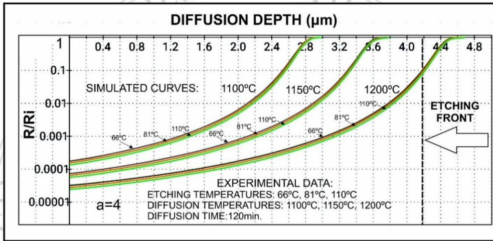
**Fig. 3.** The variation of  $R/R_i$  ratio during the chemical etching process of the boron diffused silicon layers in  $a=4$  type etching solutions, simulated according to the analytical results describing the boron profile after the diffusion from a BN source at 1100°C, 1150°C and 1200°C for 120min. The temperatures of the etching solutions are: 66°C, 88°C, 110°C.
