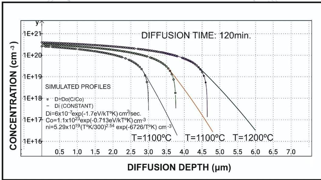
**Fig. 2.** Boron diffusion profiles in silicon simulated according to the analytical results after the boron diffusion from the BN source at 1100°C, 1150°C and 1200°C for 120min.
