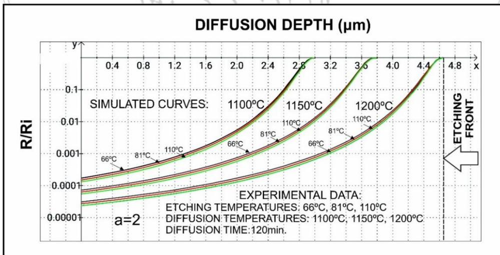
**Fig. 4.** The variation of  $R/R_i$  ratio during the chemical etching process of the boron diffused silicon layers in  $a=2$  type etching solutions, simulated according to the analytical results describing
