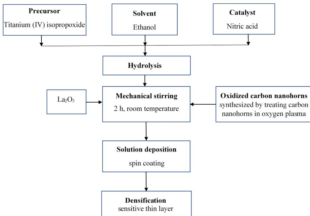
**Fig. 11.** Synthesis of TiO<sub>2</sub> / La<sub>2</sub>O<sub>3</sub> / oxidized carbon nanohorns sensing layer.
