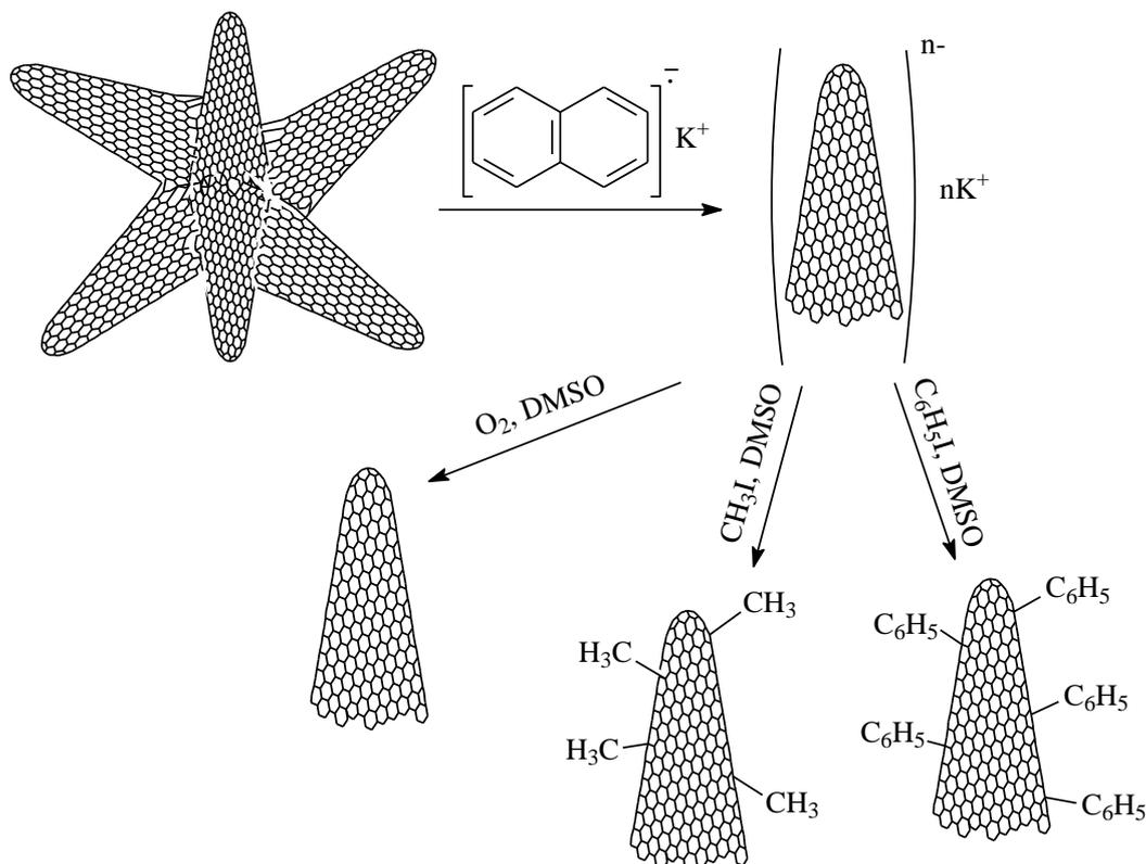
**Fig. 3.** Reductive dismantling of carbon nanohorns, reoxidation and covalent functionalization of the reduced carbon nanohorns.
