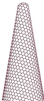
**Fig. 1.** The structure of a carbon nanohorn.
