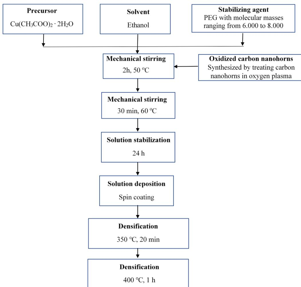
**Fig. 9.** Synthesis of CuO/ oxidized carbon nanohorns - based sensing layer using poly(2 ethyl- 2- oxazoline) as stabilizing agent.
