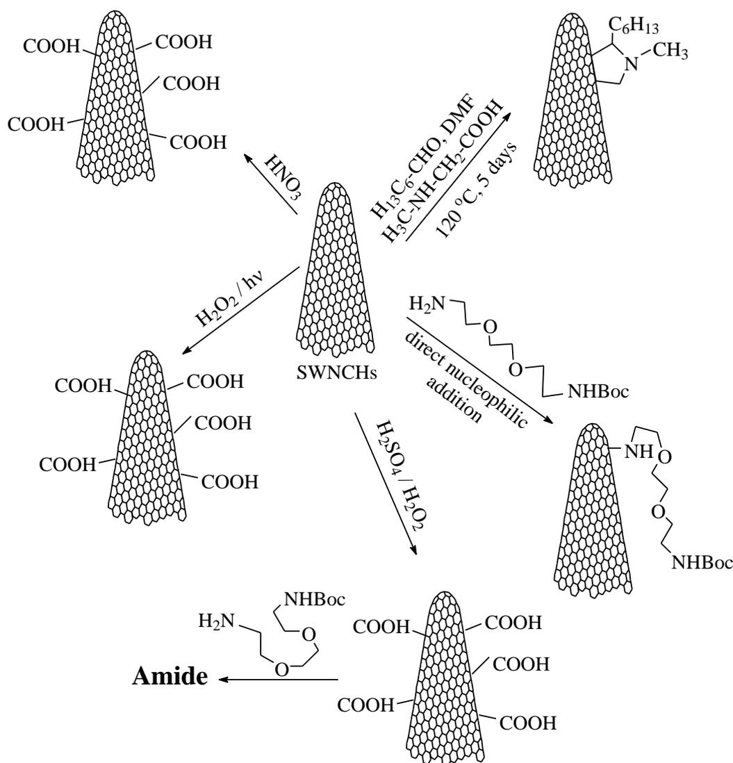
**Fig. 2.** Different types of covalent functionalization of SWCNHs.
