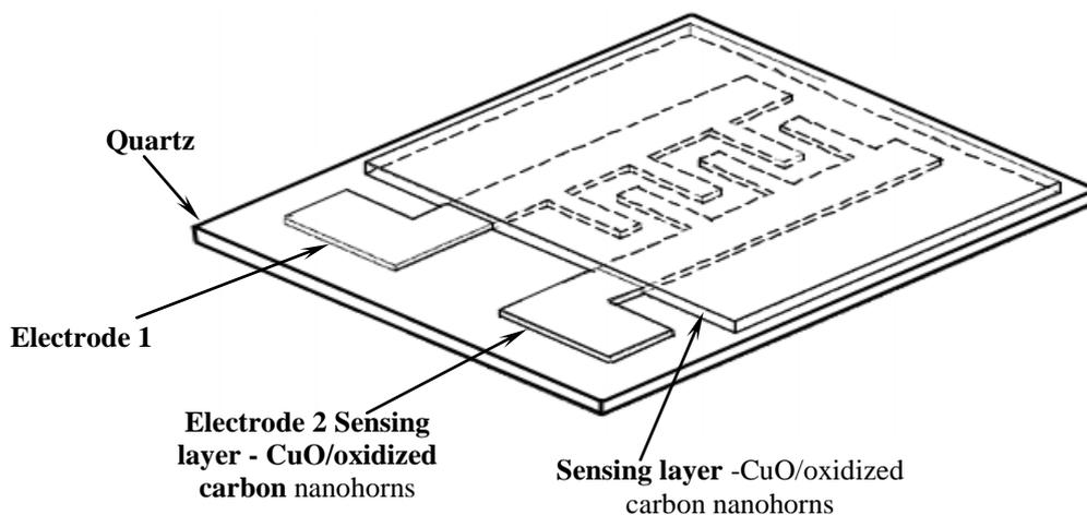
Fig. 5. The structure of the sensor with interdigitated electrodes.
