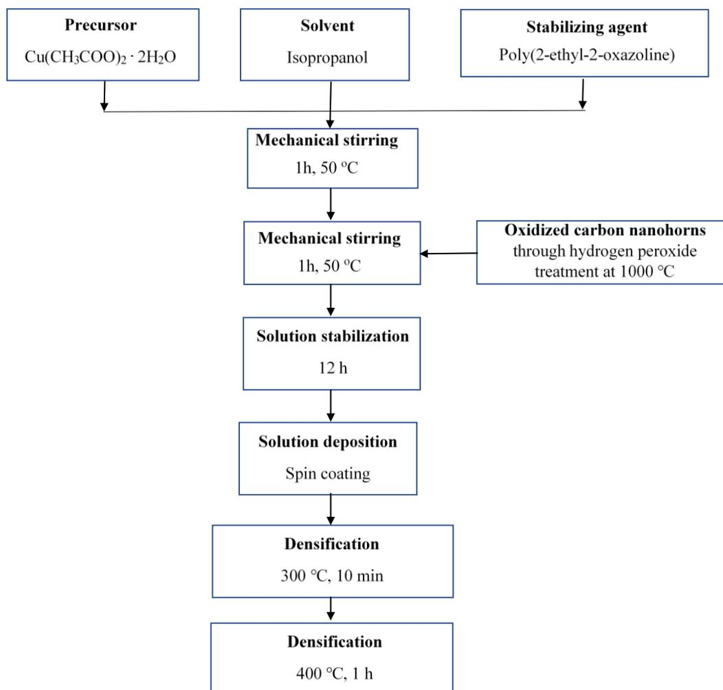
**Fig. 8.** Synthesis of CuO/ oxidized carbon nanohorns - based sensing layer using poly(2 ethyl- 2- oxazoline) as stabilizing agent.
