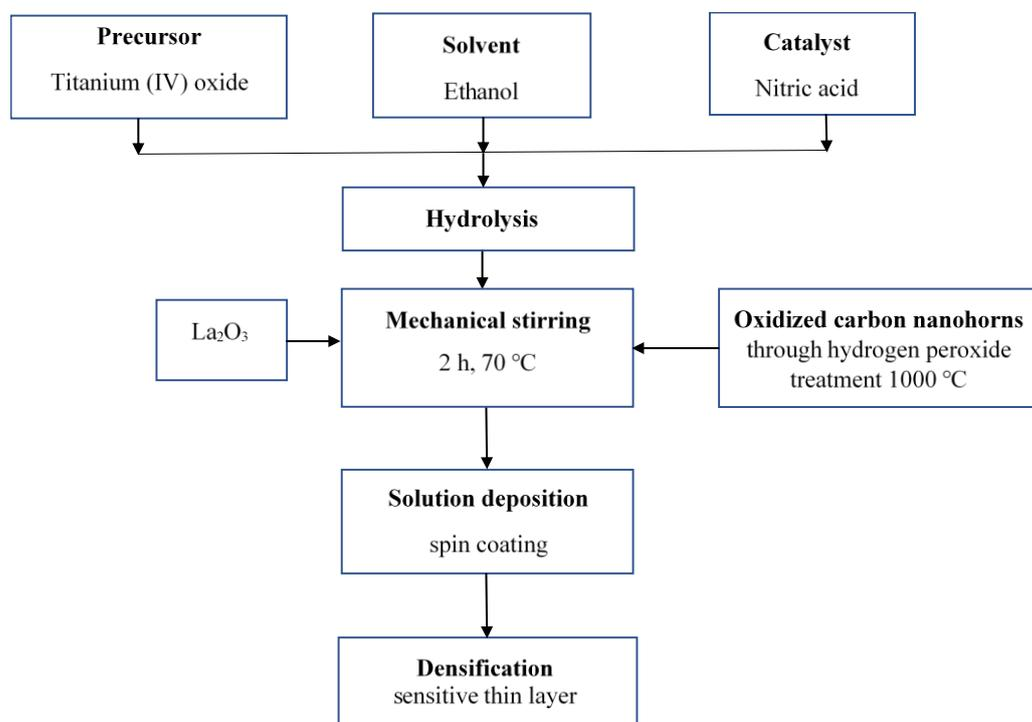
**Fig. 10.** Synthesis of TiO<sub>2</sub> / La<sub>2</sub>O<sub>3</sub> / oxidized carbon nanohorns sensing layer.
