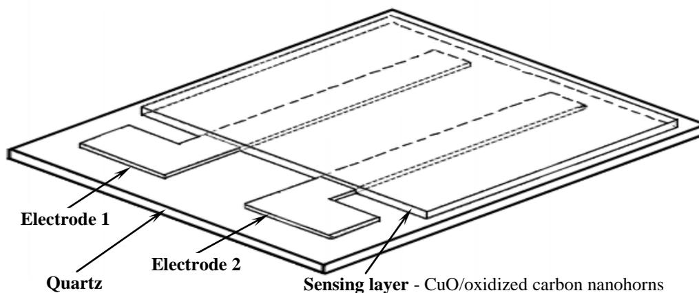
Fig. 4. The structure of the sensors with linear electrodes.
