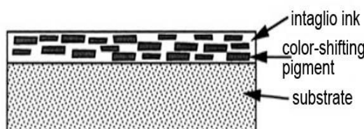
Fig. 5. Pigment ink to achieve colour variation compared to the angle of observation.
