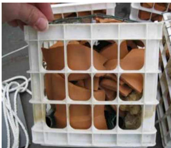
Fig. 1 - Recommended trap for sampling epifauna - collector with artificial habitat filled with: broken pots, decorative stones and pieces of rubber tubes (original photo, NIMRD).
