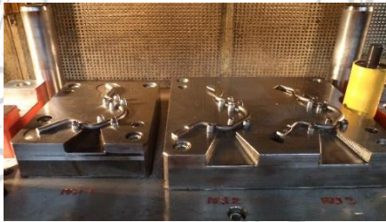
Fig. 12. The piece placed in the multi-post die
