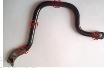
Fig. 20. Defect of painted part.
