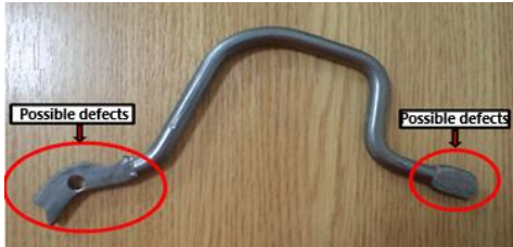
Fig. 19. Defect on the part – off - center hole and missing perforation.
