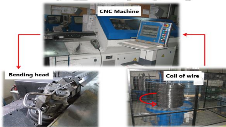
Fig. 5. Wafios bending machine & wire coil
