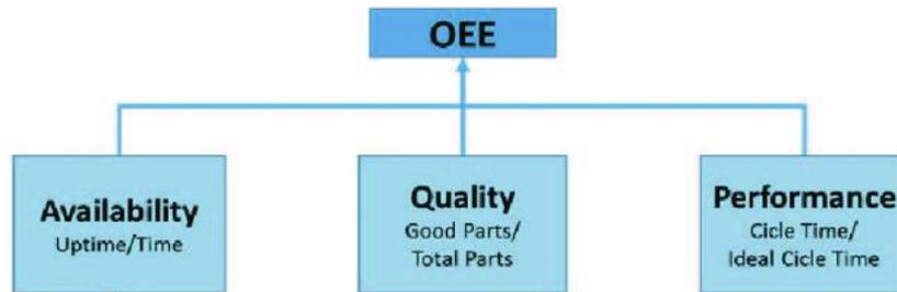
Fig 1. OEE indicator components.
