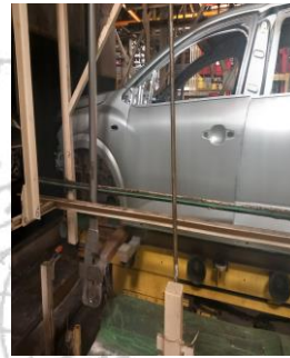
Transfer of the bodywork inside the bathroom areas TTS degreasing and cataphoresis application with the help of transport pendulums
