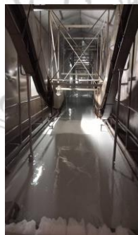
Car body washing with high-pressure spray nozzles to remove possible impurities (spray washing after each stage/bath).
