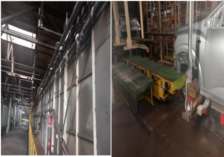
Transfer of the bodywork inside the bathroom areas TTS degreasing and cataphoresis application with the help of transport pendulums
