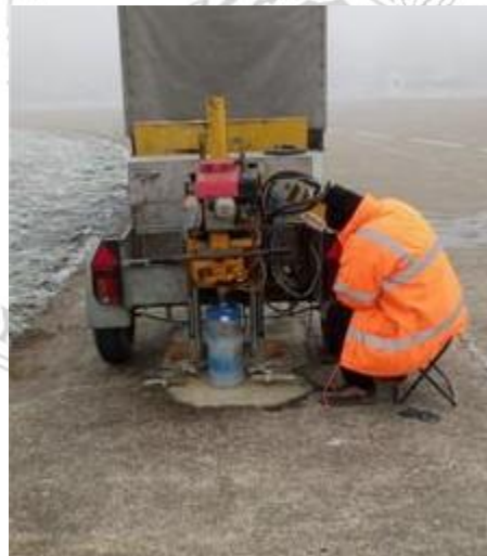
Fig. 3. Carrying samples with a diameter of 200 mm.
