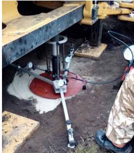
Fig. 1. Finding ground reaction modulus using LUKAS plate.
