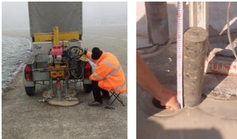
Fig. 5. Sampling of carrots with a diameter of 100 mm and their measurement.
