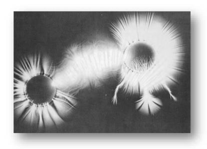
**Top cover image:** Anodic electronographic discharge at the interface between a microscope quartz slide sitting on glass electrode (gray region is quartz slide while black region is the air nearby).
