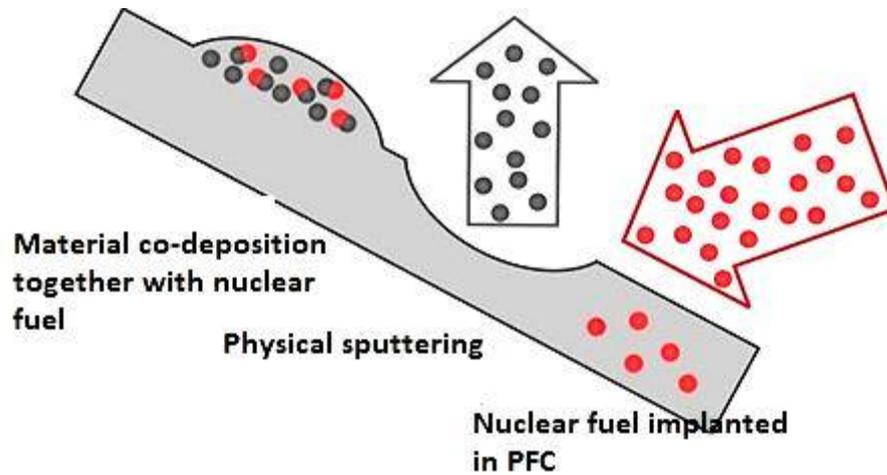
**Fig. 2.2** Schematic representation of the main processes occurring at the interaction of fusion plasma with PFC's
