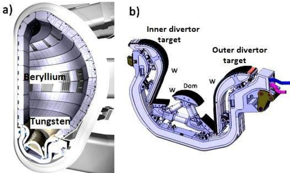
**Fig. 2.1** a) ITER chamber section b) Divertor section assembly
