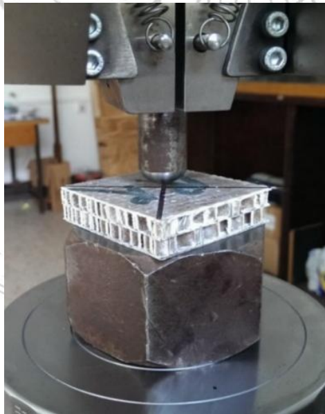
Fig. 4. Multilayered honeycomb composite material in test position.
