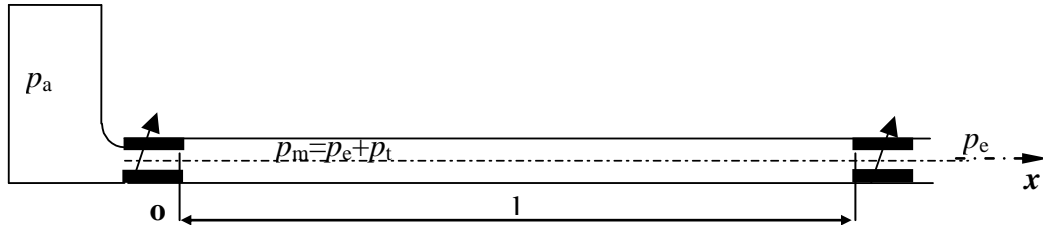
Fig. 1. A two-stage demand regulator represented as an assembly of two variable nozzles connected by a medium pressure hose.
