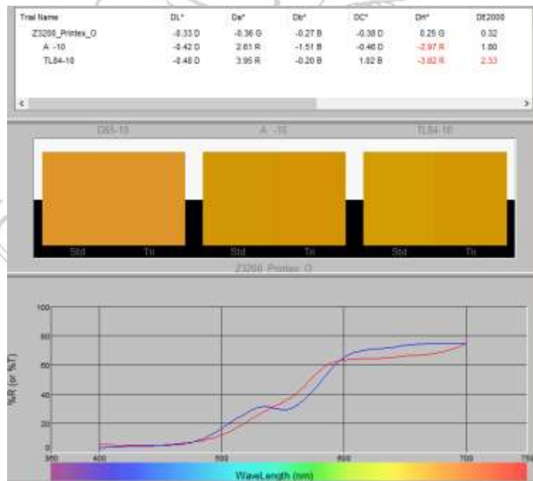
Fig. 12. \Delta E^*_{00} and MI evaluation Color Standard/Reproduction Sample.
