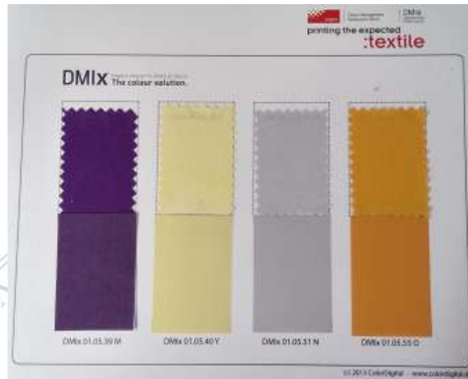
Fig. 11. Side-by-side view of master color standards and digital prints reproductions under reference conditions.
