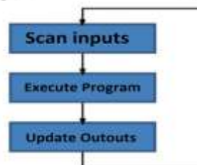
Fig. 11. Basic PLC Program execution cycle.
