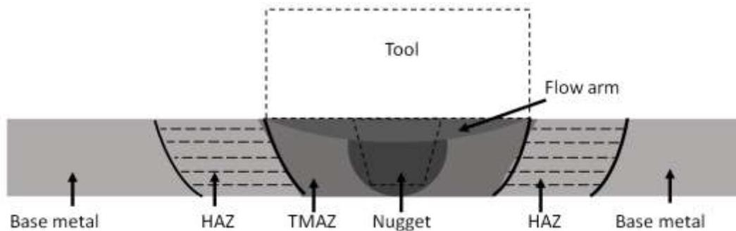
Fig. 2. Decomposition of the welded zone.
