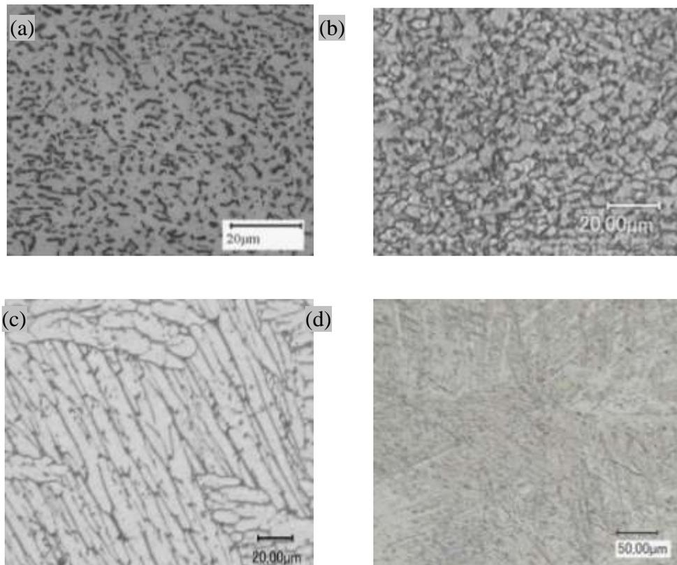
**Fig. 3.** Different microstructures obtained: (a) fine equiaxe, (b) duplex, (c) coarse lamellar, (d) fine lamellar.
