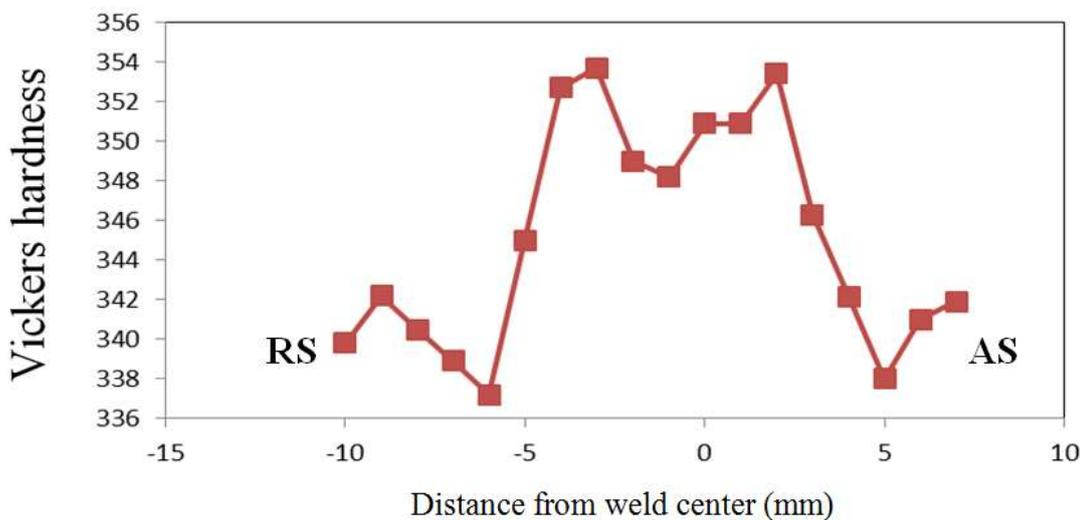
**Fig. 4.** Hardness profile in a sample welded in condition 1.
