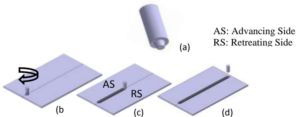
**Fig. 1.** Representation of the FSW process: (a) FSW tool
