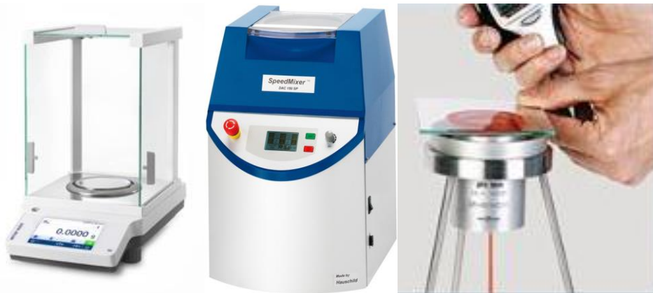
Fig. 3. Operation of analytical balance, ink speed mixer and flow cup.
