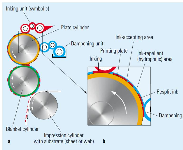
**Fig. 1.** Components of a printing unit.
