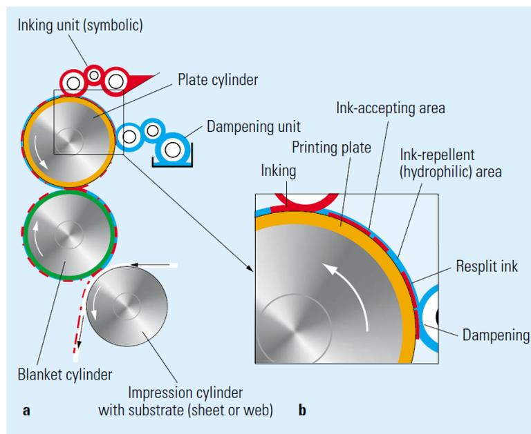
**Fig. 1.** Components of a printing unit.
