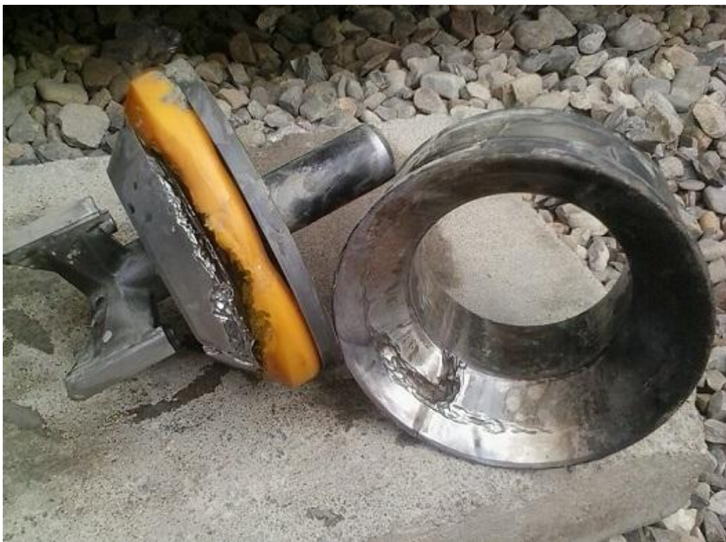
Fig. 4. Valve components (valve body, valve insert, valve seat) affected by erosive wear.
