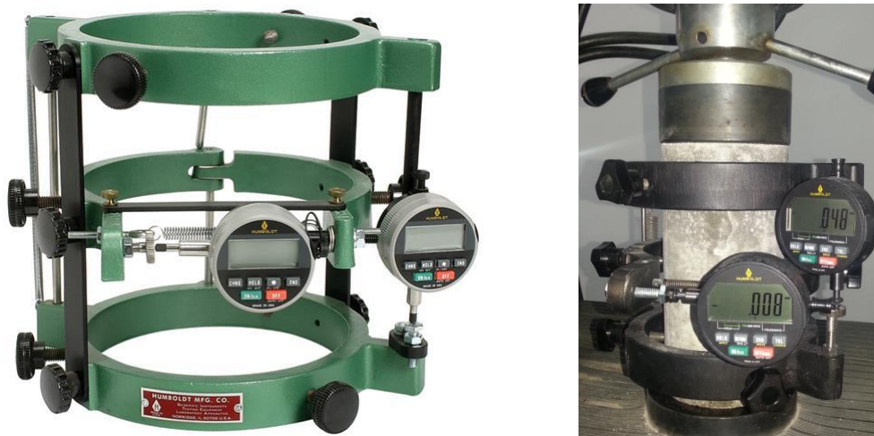
Fig. 1. Determination of the modulus of elasticity in compression.
