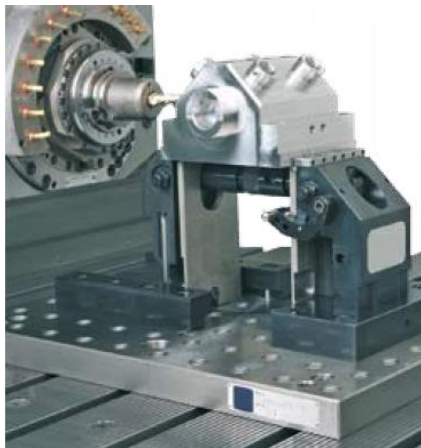
Fig. 3.1. Modular clamping system [13].
