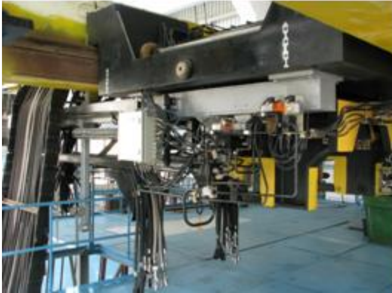
Fig. 4. F/M testing rig: bridge, carriage and catenary (partial view).
