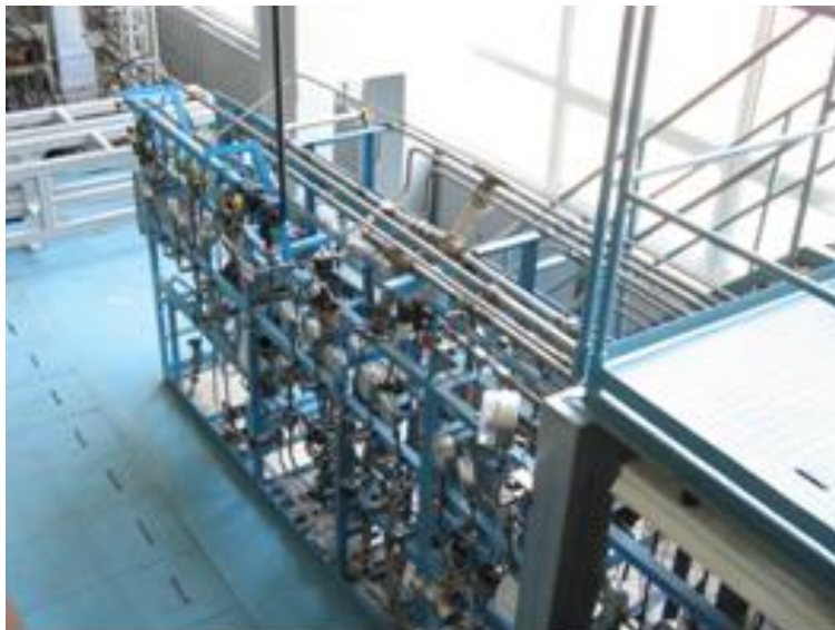
Fig. 3. F/M testing rig: valve station (partial view).
