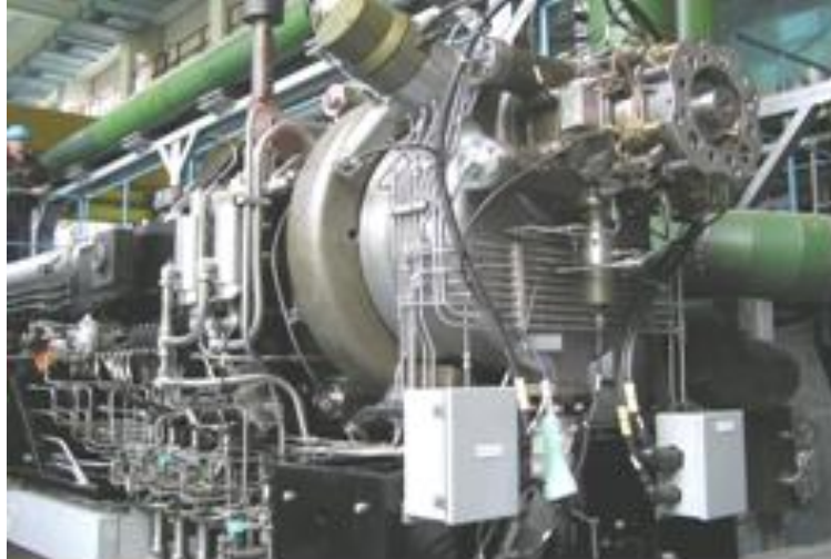
Fig. 1. CANDU 600 Fuelling Machine (partial view).
